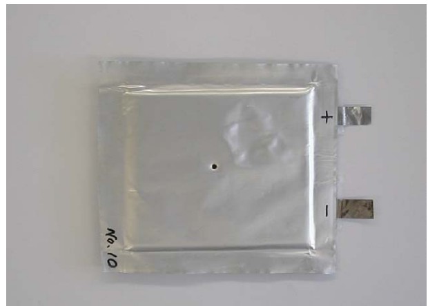
Fig. 11. Photograph of a Li-ion semi-IPN gel polymer (2500 mAh) cell after a nail penetration test.
